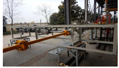
The performance of wet gas flow meter at single-phase dry gas is first tested as the base reference for the wet gas flow test. After the dry gas test, the liquid is gradually injected into the natural gas flow from less to more to conduct the wet gas flow test.
